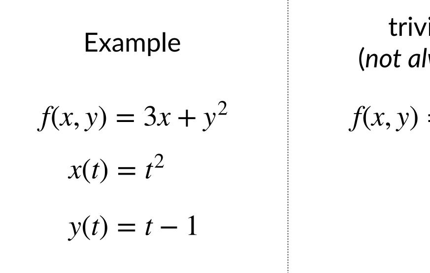
$\frac{d}{dt}f(x(t), y(t)) = \frac{\partial f}{\partial x} \cdot \frac{dx}{dt} + \frac{\partial f}{\partial y} \cdot \frac{dy}{dt}$
